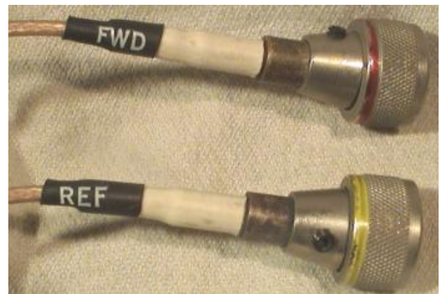
VSWR sample lines. Notice the color banding
