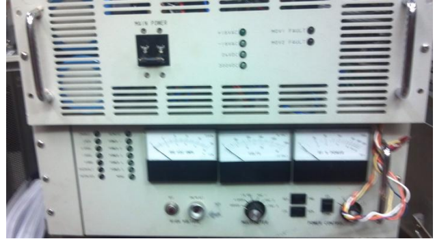
A 1 kW Omnitronix transmitter on the test bench
