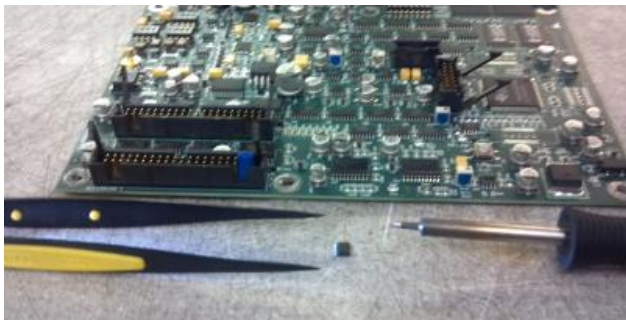
SMDs present a real challenge during repairs, as on this DAX-1 exciter board
