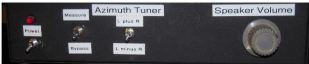
The front of my azimuth gadget. The volume control adjust on the front of the box is not necessarily related to the project – I needed a way to adjust volume between pre-amp out and power amp input and this was a convenient place to put the control.
