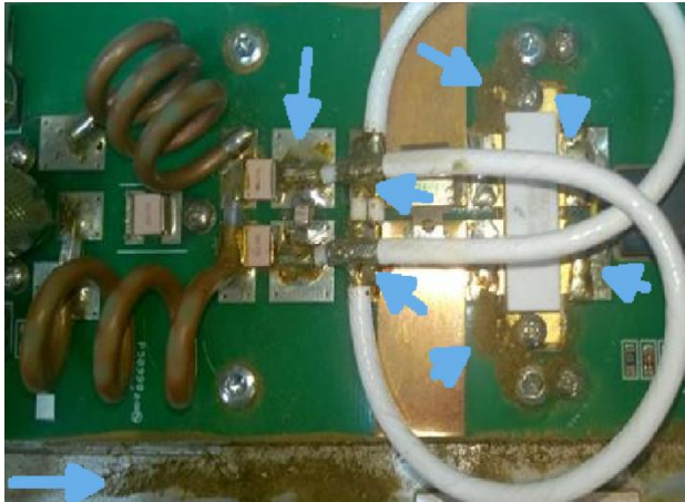
The crud accumulates!
