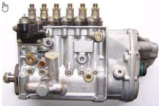
For a typical six-cylinder engine, there were six thin steel tubes from the injector pump to the
