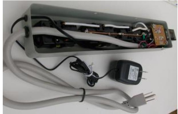
**A small circuit allows remote power resetting**
