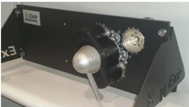
Using mechanical advantage and intricate mechanisms, even a large patch link can be moved easily with one hand and *no* tools.
