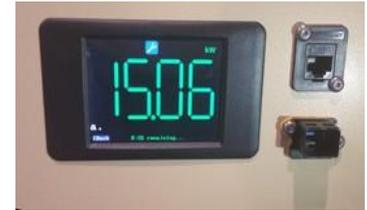
At first glance, a network-aware dummy load seems a little superfluous but, in today's SNMP-monitored broadcast plant, having a reject or dummy load's power relayed directly to an SNMP server makes perfect sense in the grand scheme of integrated big picture site monitoring.
