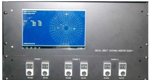
This monitor was designed with fiberoptic sample lines along with a computerized display that allows you to tweak up your phasor simply by putting the towers back where they belong.
