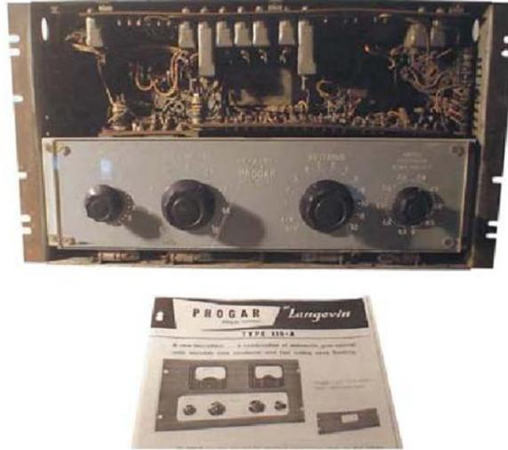
**The PROGAR brought automatic gain control and peaking limiting together.
