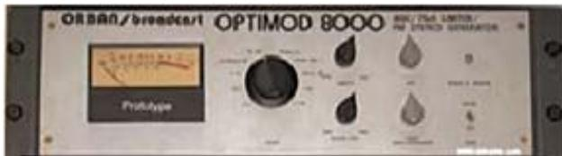
**The Optimod 8000 was the first FM processor with a built-in Stereo Generator**
