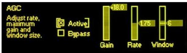
The DAVID works on a ‘windowing’ theorem, much like how the four bands in the old Texar Audio Prism worked. The result is a very smooth control of the audio input levels.
