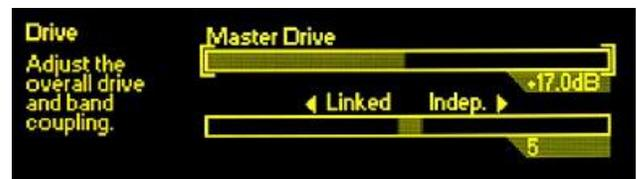
Both of these affect all five bands – you cannot, for example, increase the drive to just the mid-band. The coupling control determines the tracking between the different bands and can be set between the extremes of completely independent and completely ganged (wideband operation).
