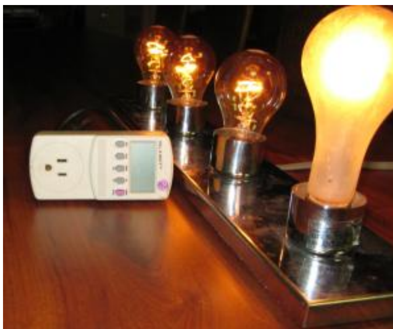
With the lamps on line, the full capacity of a UPS can be tested
