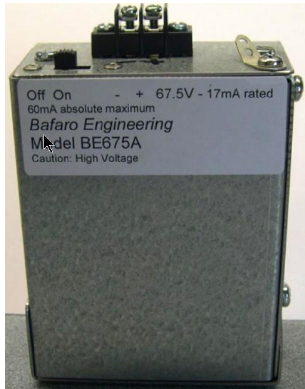
The BE675A. Note the on/off switch on the left side, to enhance the battery life.
