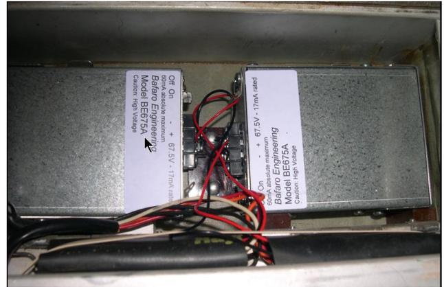
**Two BE675A modules installed in an N-C 120B to replace the two B batteries.**
