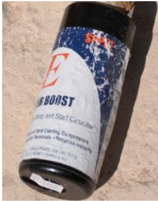
An air conditioning unit capacitor
