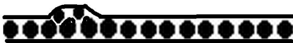
Pressing the BBs into the tube can cause the walls to buckle
