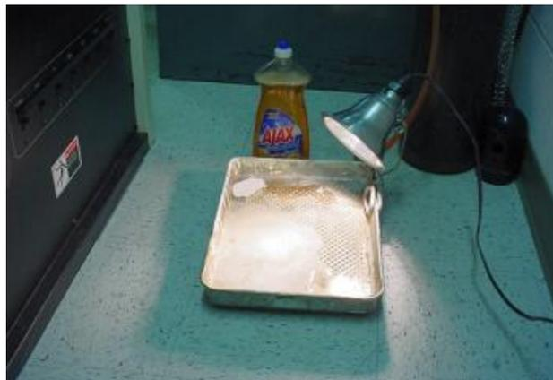
The way it works is simple. When the rest of the transmitter room is dark, the moths are attracted to and circle the light attached to the pan.
