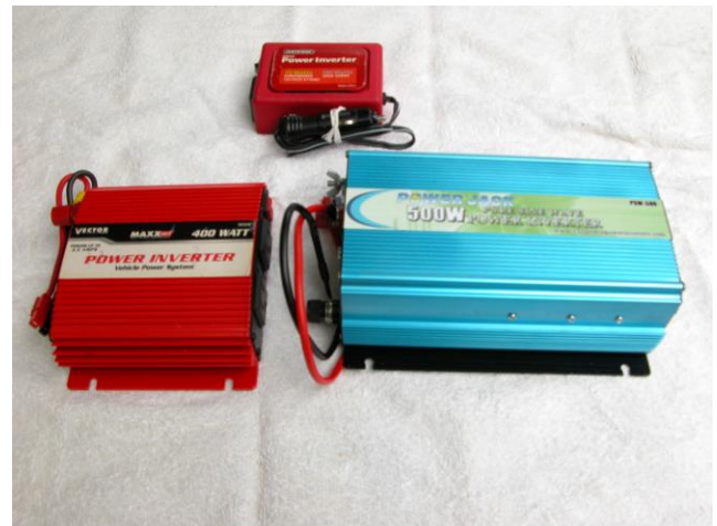
Top: Ray-O-Vac, 75 Watts, modified sine-wave Lower left: Vector, 400 Watts, modified sine-wave. Lower right: PowerJack, 500 Watts, pure sine-wave.
