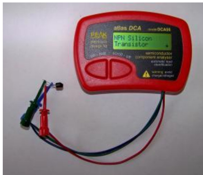
The Peak Atlas DCA55 automatically identifies the device under test.
