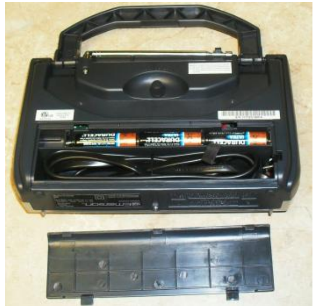
A look at the back of the Emerson RP6251. The knob on the back is for Weather Band tuning.
