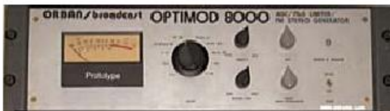
The Optimod 8000 was the first FM processor with a built-in Stereo Generator
