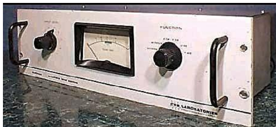
The Audimax I A straight-ahead audio compressor
