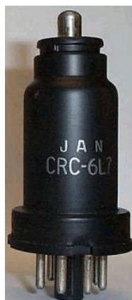
The 6L7 came in a metallic style and the 6L7G glass envelope
