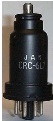
The 6L7 came in a metallic style and the 6L7G glass envelope
