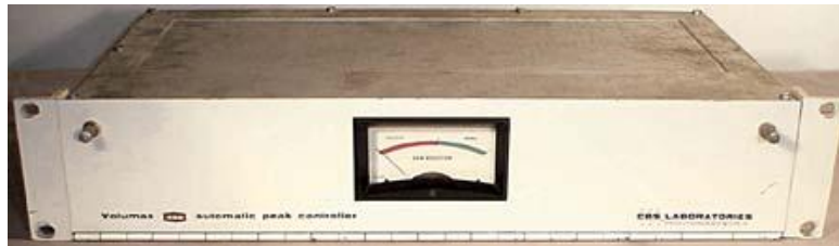
The Volumax provided a limiter to complement the Audimax
